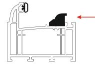
Fit a 17mm Frame Wedge to the outer frame on the stay fixing area
